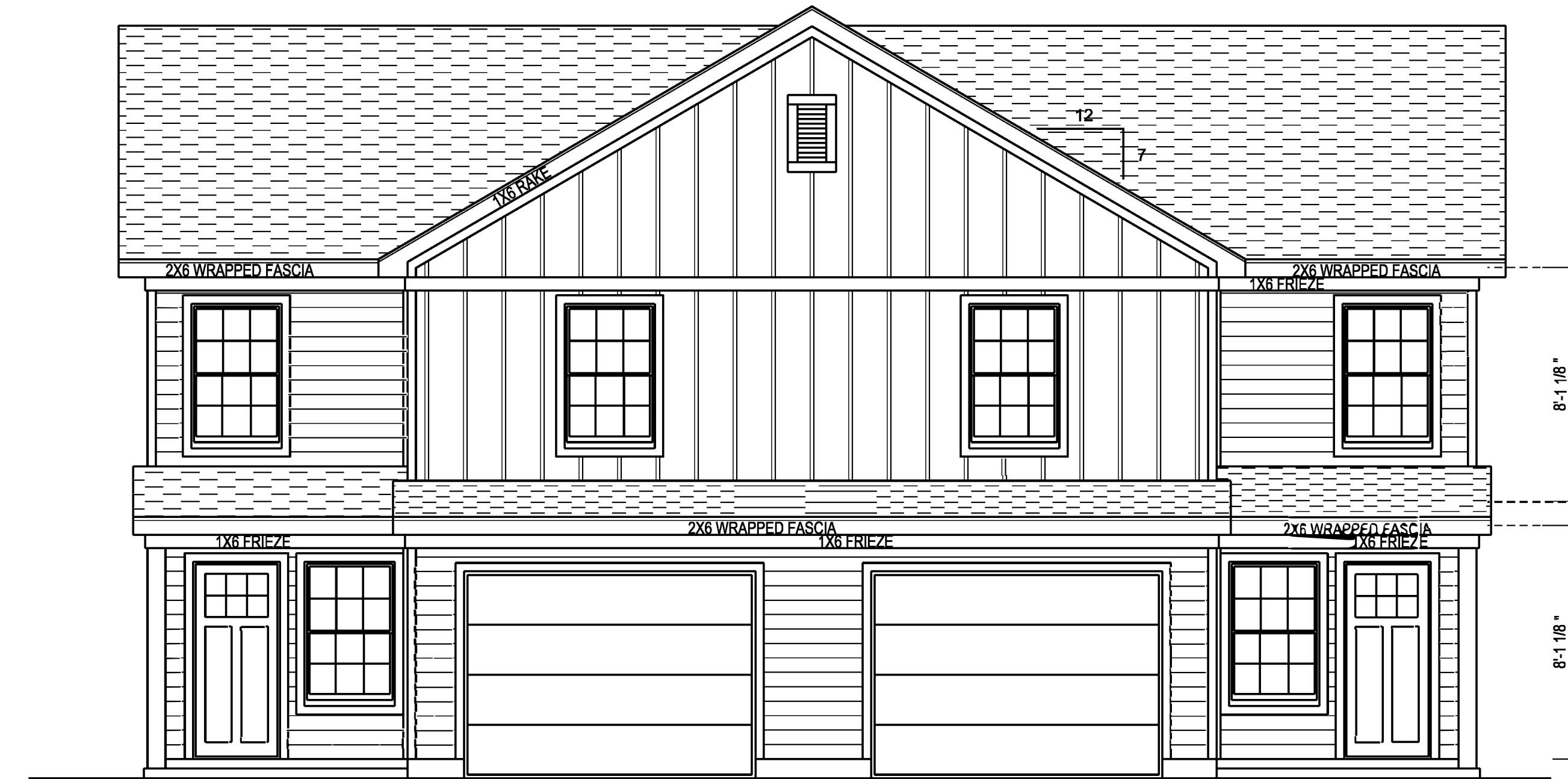
- FRONT ELEVATION - UNIT B
